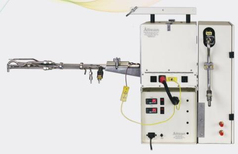
The Apex Instruments Compact Method 23 sampling system is utilized for US EPA Method 23 Determination of Dioxins and Furans from stationary sources. Dioxins and furans are an unwanted by-product of combustion processes such as municipal and industrial waste, wood and oil burning. The sample is withdrawn from the gas stream isokinetically, passed through the probe, through the filter assembly, and then through the glassware train.
