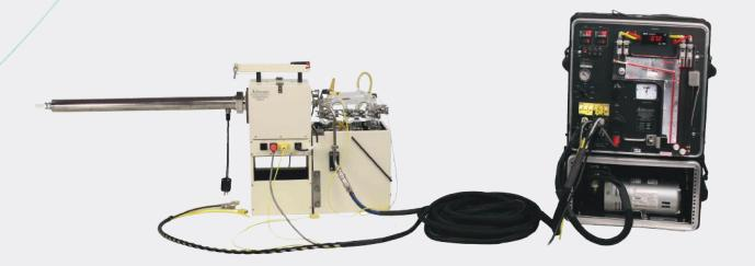
Controlled Condensate is an alternative to EPA Method 8 for determining sulfuric acid emissions. Sulfuric acid vapor or mist and the sulfur dioxide are separated by controlling the condensation based on the difference in dew points: both fractions are measured separately by the barium-thorin titration method.
