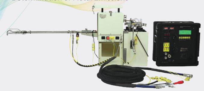
The Method 29 determination of metal emissions from hazardous waste incinerators involves a modification of the Method 5 train. The sampling train is the same as a Method 5 particulate train with the addition of up to three impingers to enhance the collection of metals of interest. The impinger train requires the SB-4 impinger case, glass nozzle and probe liner, and a non-metallic union. The method has been validated for the collection of 17 different metals.
