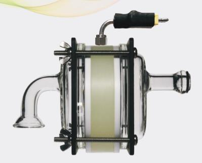
The exhaust from a wood heater is collected with a total collection hood and is combined with ambient dilution air. Particulate matter is withdrawn proportionally from a single point in a sampling tunnel and is collected on two glass fiber filters in series.
